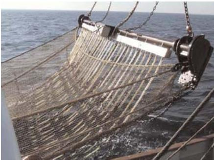
Figure 19: the pulse trawl
