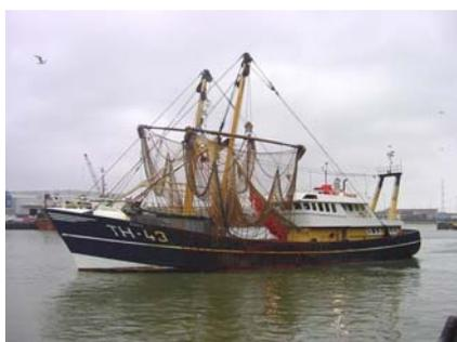
**Figure 7: cutter with beam-trawl nets**
